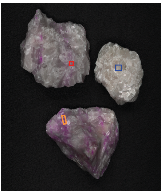
False colour display of calcite samples with ROI markers; acquired with BlackIndustry SWIR 1.7 Pro Max
